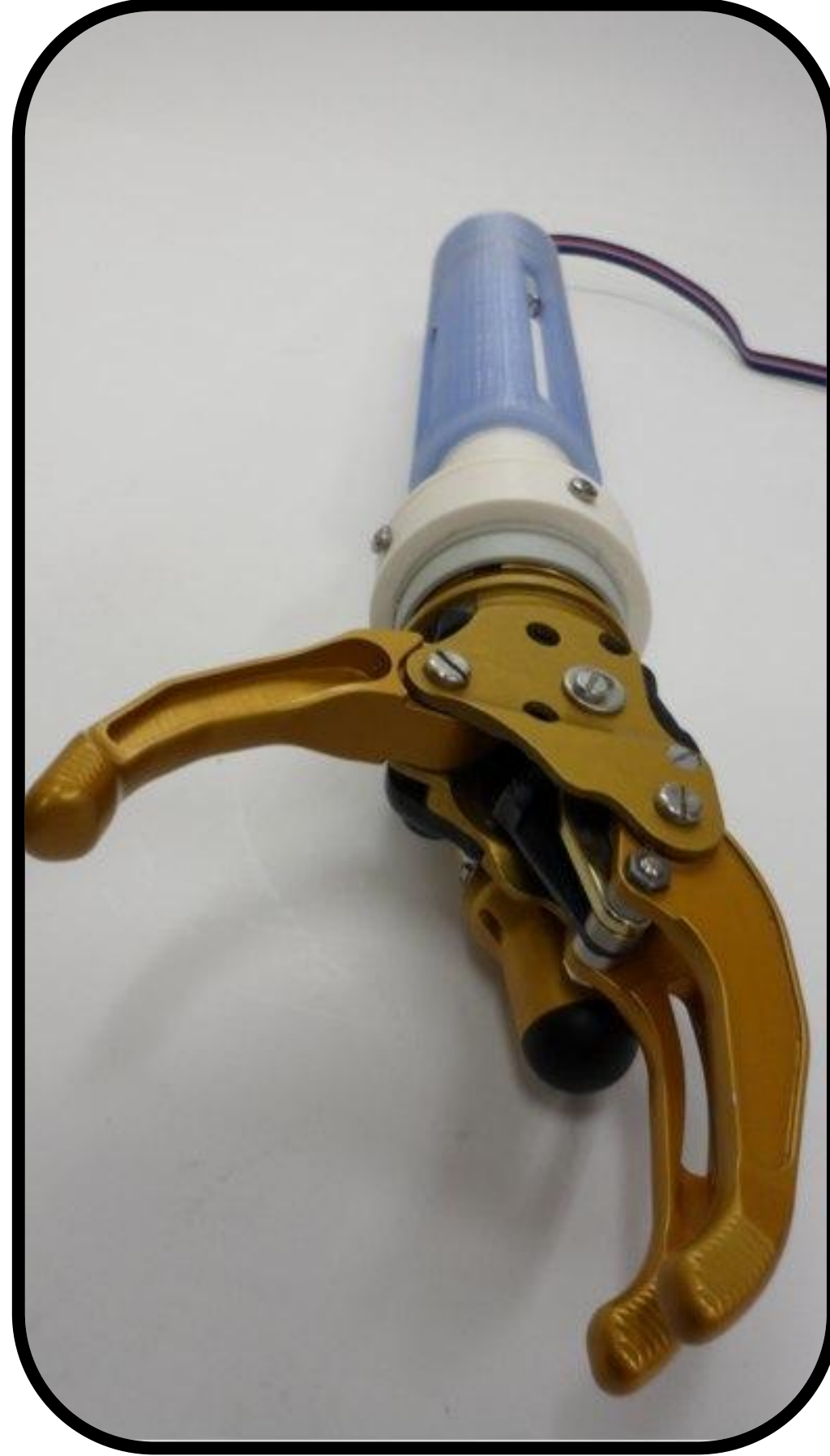
Extendable Forearm Prosthesis (a.k.a. the "Go-Go-Gadget Wrist")
